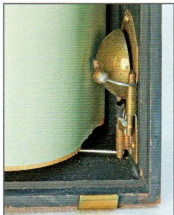
Bell inside the 1892 No. 5 Folding Kodak roll holder. After one rotation of the measuring roll, the bell strikes to indicate that enough film is wound on.
