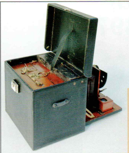
Typical amateur camera outfit at the end of the 1880's, consisting of case (for camera and plate-holders), camera and tripod. In: Photography in the studio and in the field, by E.M. Estabrooke.
