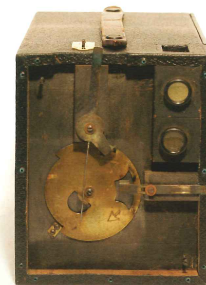
Figure 8, left. The 4 x 5 Bull's-Eye. Figure 9, right. Front side of the 4 x 5 Bull's-Eye with shutter mechanism visible. Photos by Jos Erdkamp.
