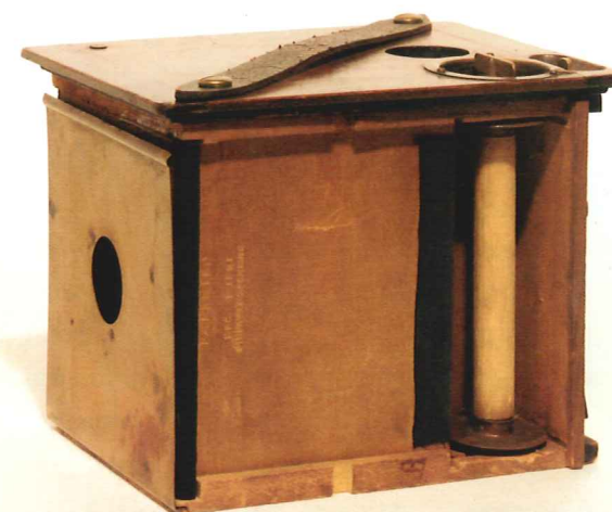
Figure 5, left. Film roll holder for the regular Bull's-Eye. Photo by Jos Erdkamp. Figure 6, right. Advertisement from American Amateur Photographer promoting three models of the Bull's-Eye.
